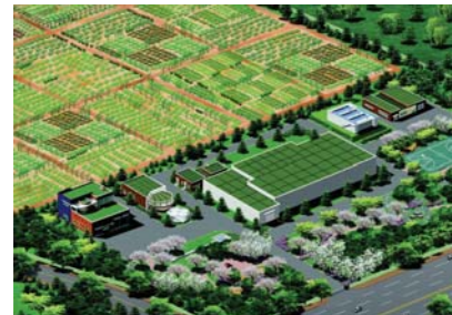
Songdo, Korea (2004) - 33 000 PE Simultaneous nitrification/denitrification after physical-chemical settling. 4 cells, 63 m 2 each
