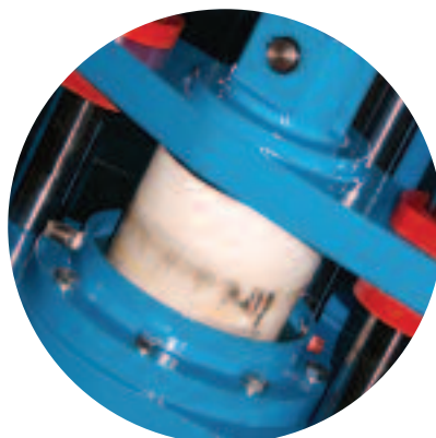
Proximity switches sense the position of the pump ram and relay this to the PLC
