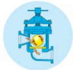
Biased flow in the ball valve housing balances out the wear on the ball thereby prolonging valve life
