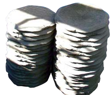
Technosand dewatered using a filter press
