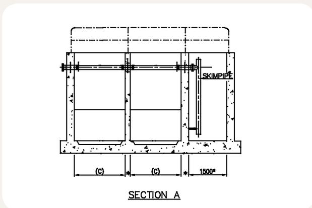
B\*: separation compartment only. The overall length (composed of inlet, oil and outlet compartment) varies upon specific customer requirements, true capacities and site conditions.
